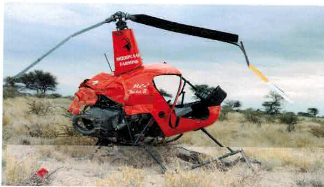
Figure 1. A photo showing the aircraft where it crashed after it struck a single phase electrical cable, the tail rotor system was cut off completely, the cockpit wind shield has shattered, the right landing skid is broken and the main rotor blades are broken into pieces due to impact forces with the aircraft structure and the ground.
