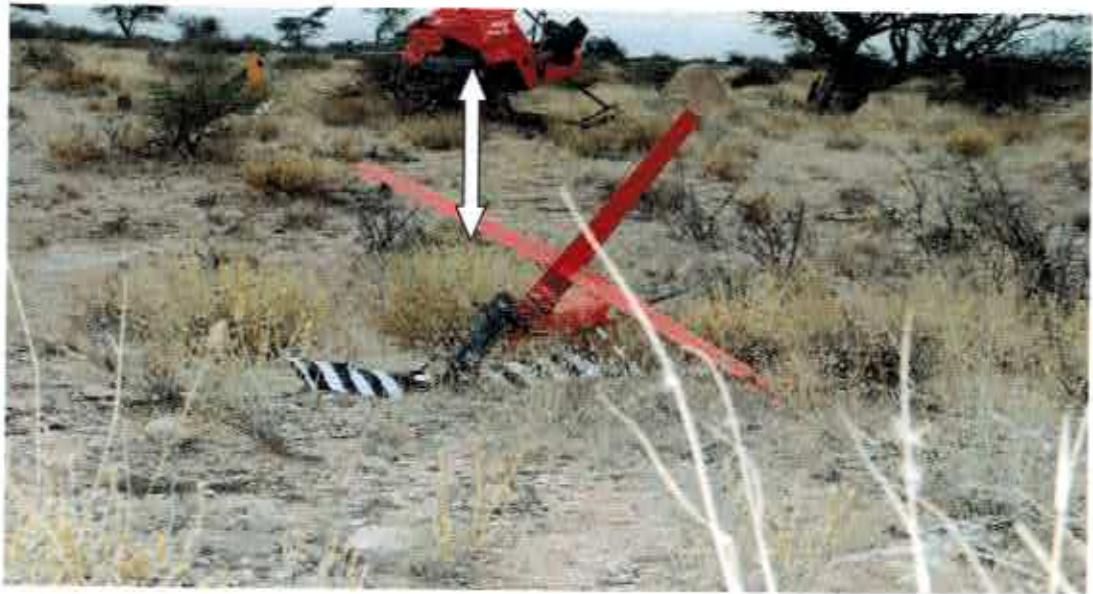
Figure 3. A photo showing the tail rotor system 33.1 metres away from the main wreckage
