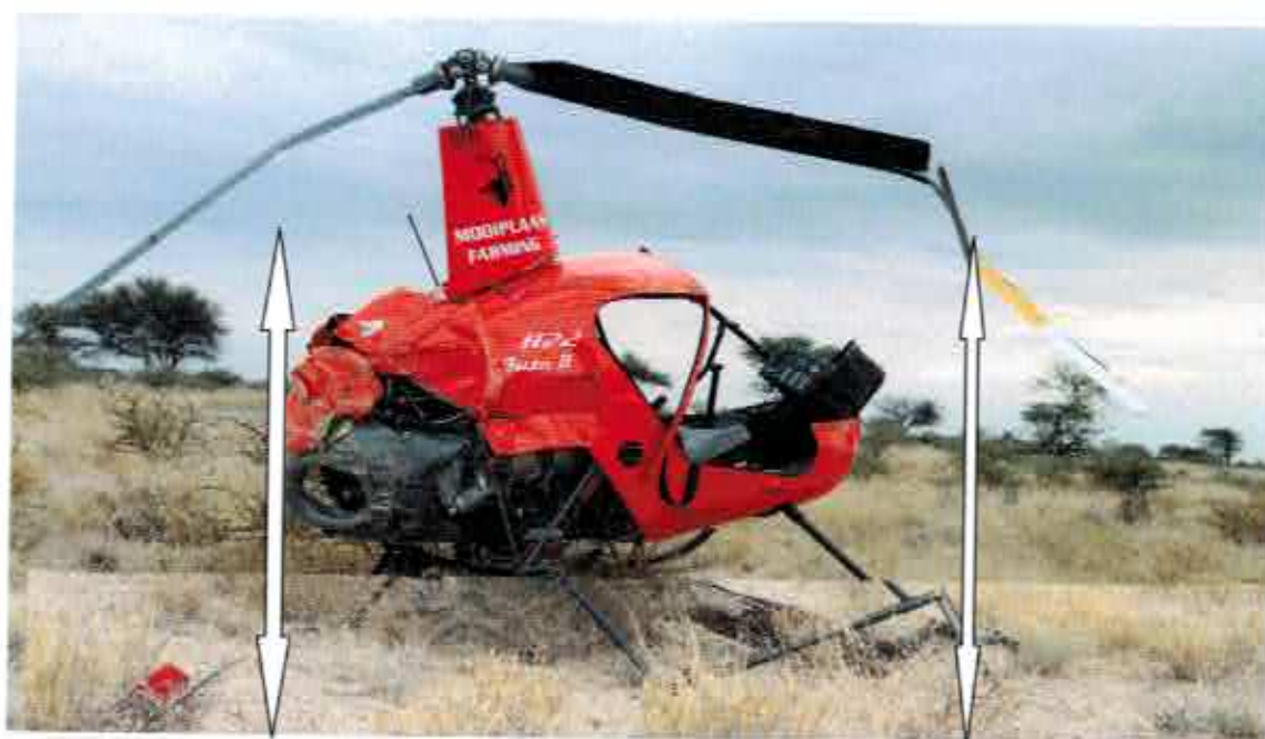
Figure 2. This photo shows the electrical cable that the aircraft struck and damages on the air frame and rotary system.
